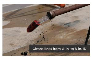
Controlled-Volume Pigging (CVP) is a highly effective pipe and tube cleaning method that outperforms flex lancing, hydro blasting and conventional pipe pigging. It uses engineered cleaning pigs propelled by water with precisely controlled volumes, pressures and flow characteristics. The process safely removes the toughest materials from the full circumference and length of a line in a fraction of the time required by other methods.
